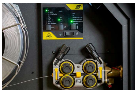
Best in class wire feeding mechanism
